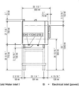
Cold Water inlet 1 CWI2 Cold Water Inlet 2 D Drain
